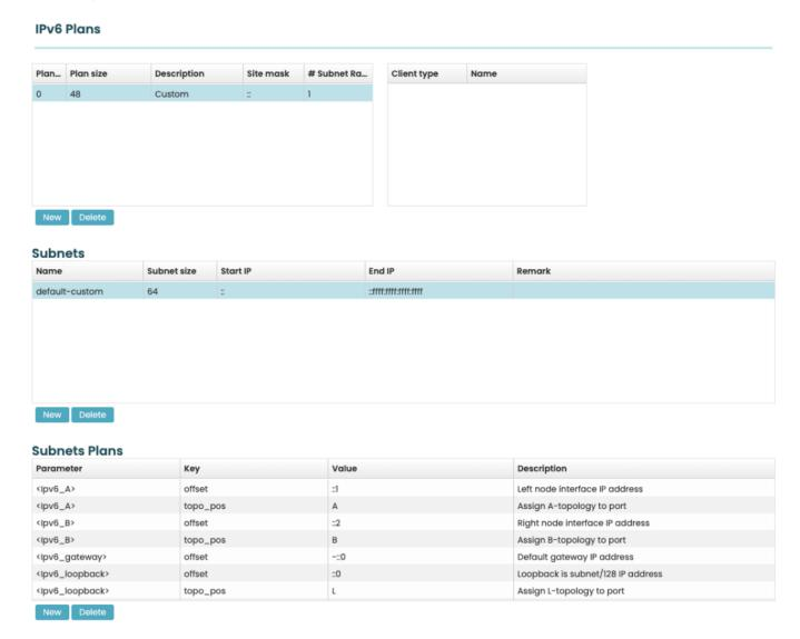
Within the current version of netYCE both **3** IPv4 and **3** IPv6 are supported. This page details the creation of IPv6 plans.
